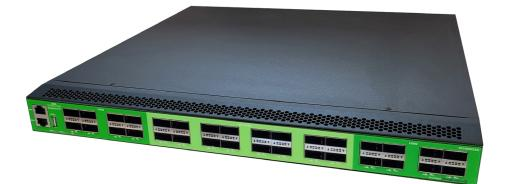
PacketMAX<sup>TM</sup>: Advanced Features are part of Garland Technology's purpose-built network packet broker lines. These Advanced Features appliances are built to extend the feature set of any product. The system is designed to support NTP time stamping, packet slicing, traffic aggregation, GRE Tunneling, hash-based load balancing, and deduplication. Adding these features to your existing infrastructure, can significantly reduce the processing overhead from security or monitoring tools.
