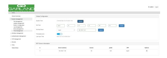
Additional NTP Servers may be applied by repeating Steps 4 and 5. The first NTP server added will be the highest priority, #1. Additional NTP servers added will be #2, #3 etc.
