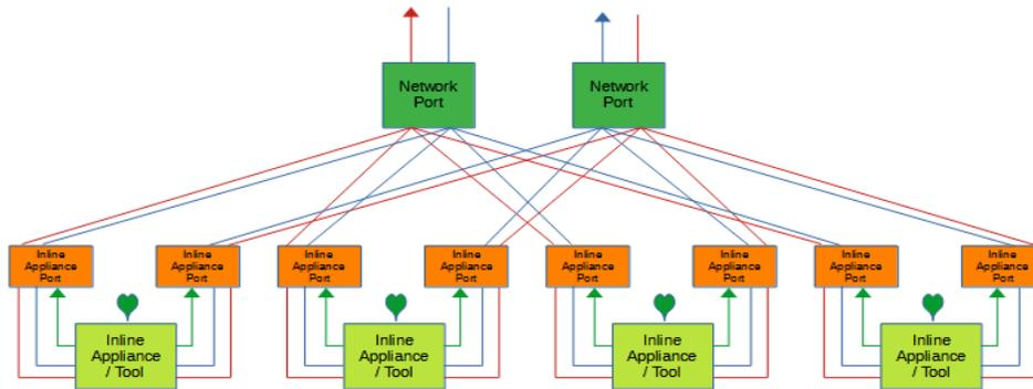
Figure 19 Load Balance Tap Mode (Bypass, Bypass Threshold=2)
