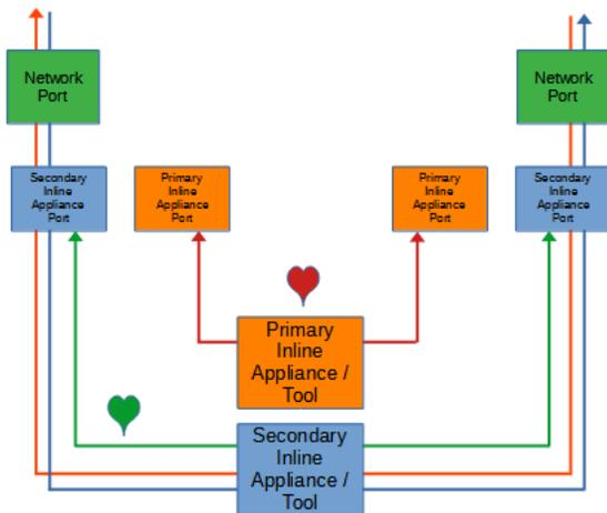
Figure 10 Primary-Secondary Tap Mode (Primary Inline)
