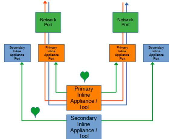
Figure 12 Primary-Secondary Tap Mode (Bypass)
