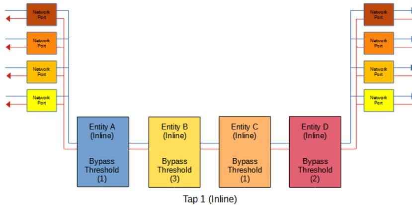
Figure 26 ATLB2 Chained Tap Mode (Bypass)
