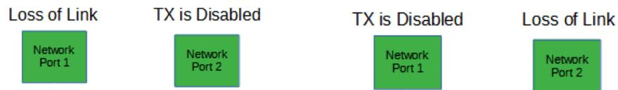
If a link is lost on one of the network ports. The TX will be disabled on the other network port. The RX for both network ports remain on.
