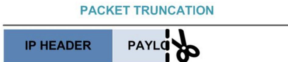
Figure 2-1 sketch map of packet truncation
