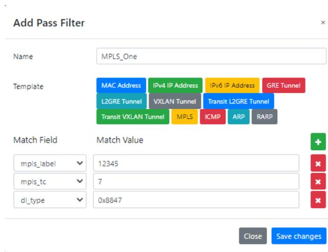
4. Select the MPLS template. When MPLS is selected the pass filter will automatically display the required options; mpls\_label, mpls\_tc and dl\_type. The dl\_type is already defined as 0x8847.
