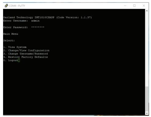
Selecting 1 brings up the View System page. This page informs the user as to the status of the power supplies and ports in addition to displaying the serial number of the unit.
