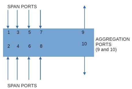
**Note:** There is no connection between ports 1 and 2, 3 and 4, 5 and 6, 7 and 8 in Span Mode. Ports can be aggregated to either ports 9 or port 10 or both,
