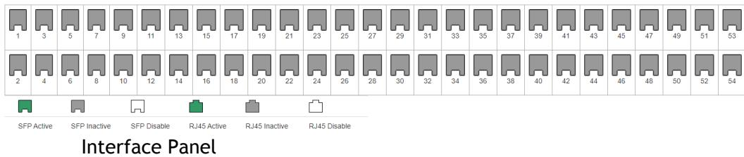
The ports on the page correspond to the actual physical ports on the switch, while distinguishing between optical and electrical ports. The status of the port is distinguished by the color of the picture, including “active”, “inactive”, “off”.
