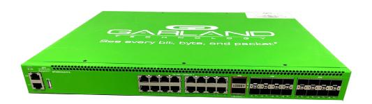
PacketMAX™: Advanced Features are part of Garland Technology's purpose-built network packet broker lines. These Advanced Features appliances are built to extend the feature set of any product. The system is designed to support NTP time stamping, packet slicing, traffic aggregation, GRE Tunneling, hash-based load balancing, and deduplication. Adding these features to your existing infrastructure, can significantly reduce the processing overhead from security or monitoring tools.
