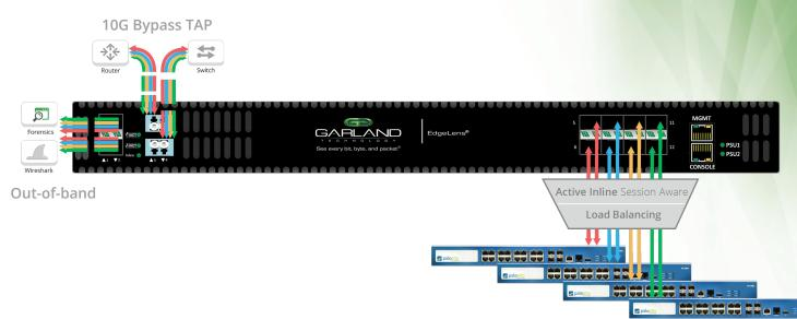
Active In-Line Load Balancing to multiple 1G Palo Alto Network Appliances
