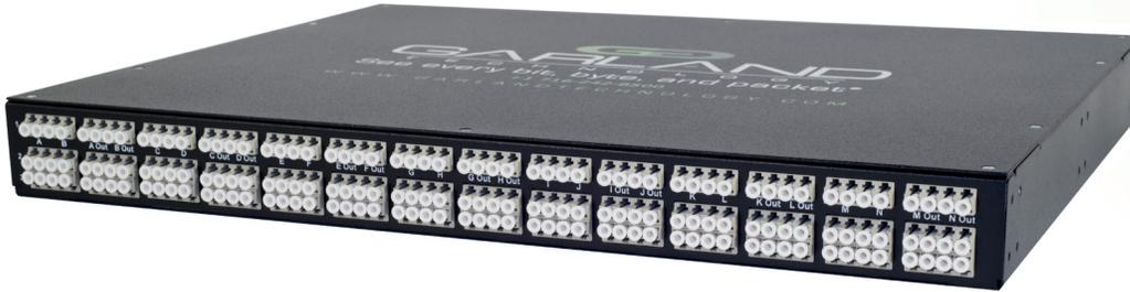
Network test access points (TAPs) are hardware tools that allow you to monitor your network. All fiber breakout TAPs are passive, purpose-built hardware devices that make a 100% copy of your network's data allowing your monitoring tools to see every bit, byte and packet.®
