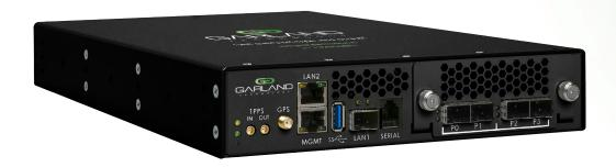
The PacketMAX™: Advanced Features Dedup is an advanced feature node, designed as a standalone platform to extend the feature set of any product. The system is designed to support large window deduplication. Deduplication can significantly reduce the processing overhead from security or monitoring tools.
