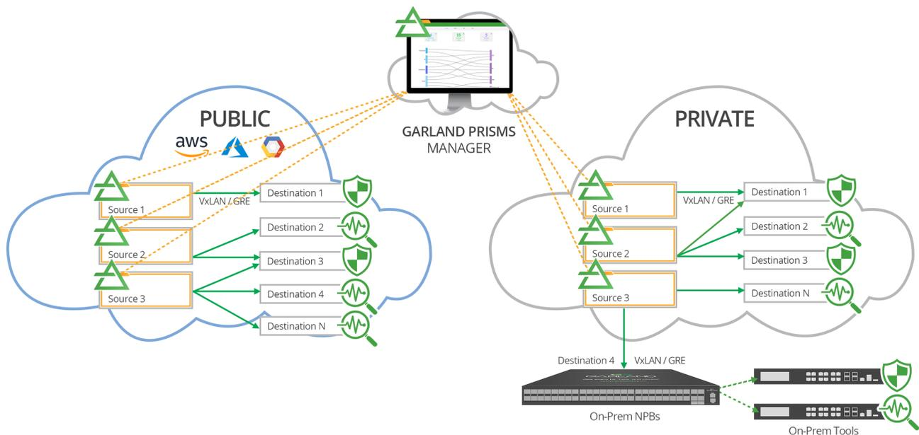
Garland Prisms virtually taps, filters and distributes cloud packet traffic to any IP address in-cloud or on-prem.
