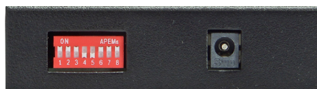
Back view of portable TAP with manual management.
