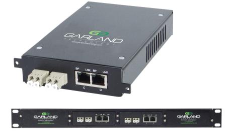
Network test access points (TAPs) are hardware tools that allow you to access and monitor your network. Aggregating TAPs are used to capture 100% full duplex traffic; the traffic can then be sent to multiple monitor appliances to analyze your network. Aggregating TAPs are purpose-built hardware devices that let you see every bit, byte and packet.<sup>®</sup>
