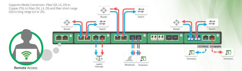
Historical Lookback (before & after) Solution with Filtering, Aggregation and Bypass with 2U - 12 TAP Modules; supports 1Gbps TAPs in columns 1, 2, 3 are deployed independently for TAP/breakout mode, aggregation and filtering with out-of-band monitoring tools. TAPs in column 4 are providing a before and after view of packets as they pass from router to forensics to active, inline security and back to forensics - before exiting through the switch.
