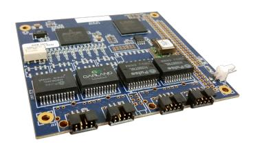
Network test access points (TAPs) are hardware tools that allow you to monitor and access your network. Aggregating TAPs are used to capture 100% full duplex traffic; the traffic can then be sent to multiple monitor appliances to analyze your network. Aggregating TAPs are purpose-built hardware devices that let you see every bit, byte and packet. ®
