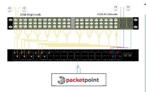
**Solution**: Prepaid Wireless Group deployed Garland Technology's SelectTAP™ using 40G passive fiber TAPs and a PacketMAX™: 100G Advanced Aggregator with breakout cables feeding into Cirries' PacketPoint, packet capture appliances 4x 10G ports.
