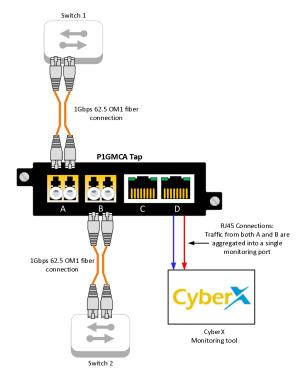
**Solution**: This utility company accomplished this with Garland Technology's 1G AggregatorTAP: Fiber, which features aggregation, regeneration and breakout TAP capabilities. The TAP will collect the data in both directions between the switches and send it out a single monitoring port to feed the CyberX monitoring software, one of the most widely-deployed ICS, SCADA & OT security platforms for effective industrial cybersecurity.
