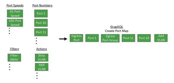
A benefit to using API's is that you could potentially make use of a monitoring tool's existing centralized management platform to also manage the Advanced Aggregators. This could allow port maps and filters to be setup on multiple appliances without having to manually access or navigate through the Aggregator's web GUI.
