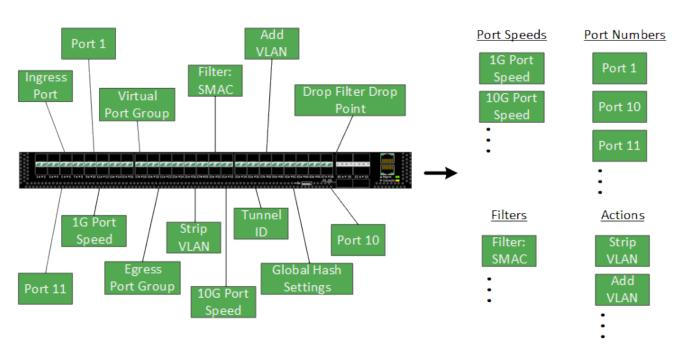
An API takes the features and capabilities of the Advanced Aggregator and makes them easily referenceable to developers that want to make use of them without having to learn and utilize the direct commands of the appliance's OS.
