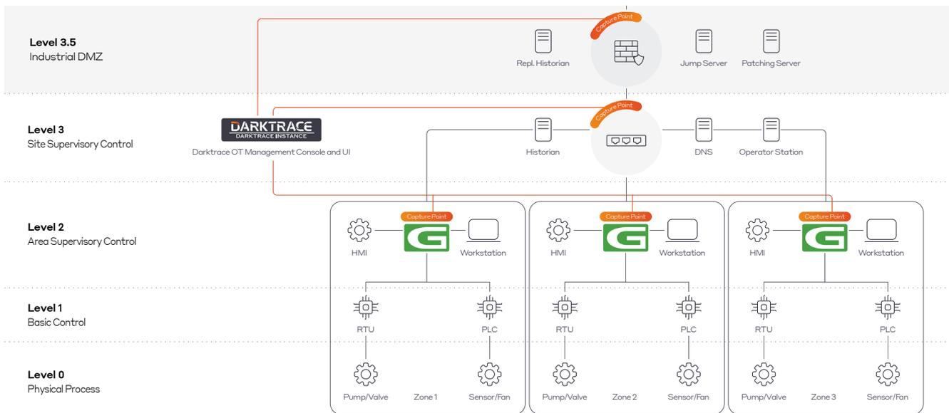
**Figure 1:** Where switching infrastructure may not exist or support port mirroring Garland taps can be used to facilitate Darktrace's passive traffic analysis
