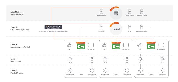
Figure 1: Where switching infrastructure may not exist or support port mirroring Garland taps can be used to facilitate Darktrace's passive traffic analysis
