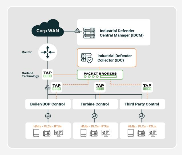
**Garland Network TAPs:** Analyze data from OT networks by mirroring network traffic. The tapped traffic can then feed into the Network Packet Broker, which combines, filters, and load balances the tapped traffic at scale into the Industrial Defender IDC data collector and/or management system.
