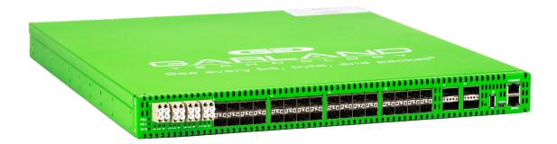
Garland Technology's Network Packet Broker without Passive TAPs is a full featured packet broker with eight (8) fixed ports (either 1G-SX/10G-SR MMF or 1G-LX/10G-LR SMF). It supports network speeds of 1G, 10G, and 40G. The fixed ports utilize internal optics with either Single Mode or Multimode connectors on the faceplate giving you the capability to connect to fiber environments. There are (32) SFP+ 1G/10G ports and (4) QSFP+ 40G ports. The QSFP+ ports can be 4x10G as well.
