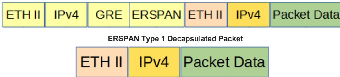
Decapsulating the ERSPAN Type 1 header from a packet(s) involves two configuration procedures.
