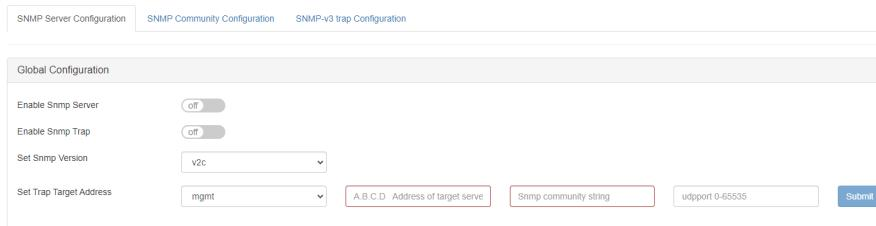
The screenshot shows the 'Global Configuration' section of the SNMP Server Configuration tab. It includes fields for 'Enable Snmp Server' (off), 'Enable Snmp Trap' (off), 'Set Snmp Version' (v2c selected), 'Set Trap Target Address' (mgmt selected), 'A.B.C.D Address of target serve' (A.B.C.D), 'Snmp community string' (snmpcommunitystring), and 'udpport 0-65535'. A 'Submit' button is at the bottom right.
