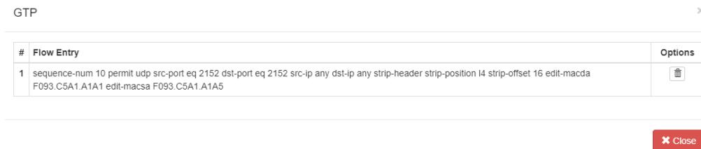
A screenshot of a software interface titled "GTP". Below the title is a table with a single row labeled "# Flow Entry". The row contains the number "1" and a detailed flow entry rule: "sequence-num 10 permit udp src-port eq 2152 dst-port eq 2152 src-ip any dst-ip any strip-header strip-position l4 strip-offset 16 edit-macda F093.C5A1.A1A1 edit-macs F093.C5A1.A1A5". To the right of the table is an "Options" column with a trash can icon. At the bottom right of the panel is a red "Close" button.
