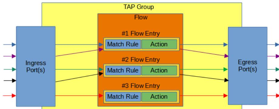
As shown in Figure 2, the entry match rule options are considered by the system as “and” options. Meaning for traffic to be permitted or denied, it must match all defined filtering options.
