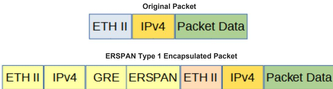
Encapsulating a packet with an ERSPAN Type 1 header involves two configuration procedures.
