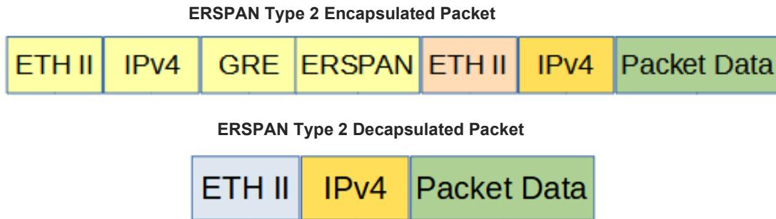
Decapsulating the ERSPAN Type 2 header from a packet(s) involves two configuration procedures.
