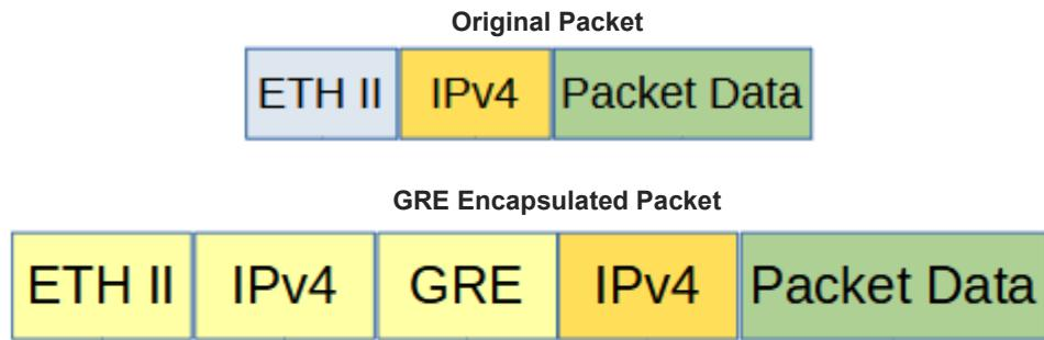
Encapsulating a packet with a I3GRE header involves two configuration procedures.
