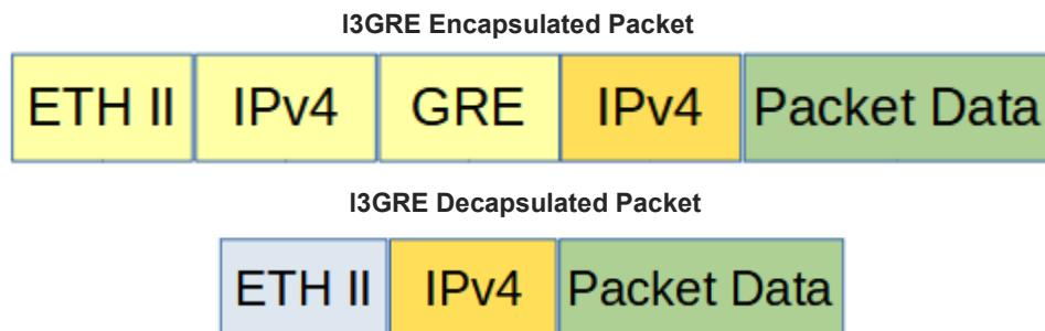
Decapsulating the I3GRE header from a packet(s) involves two configuration procedures.
