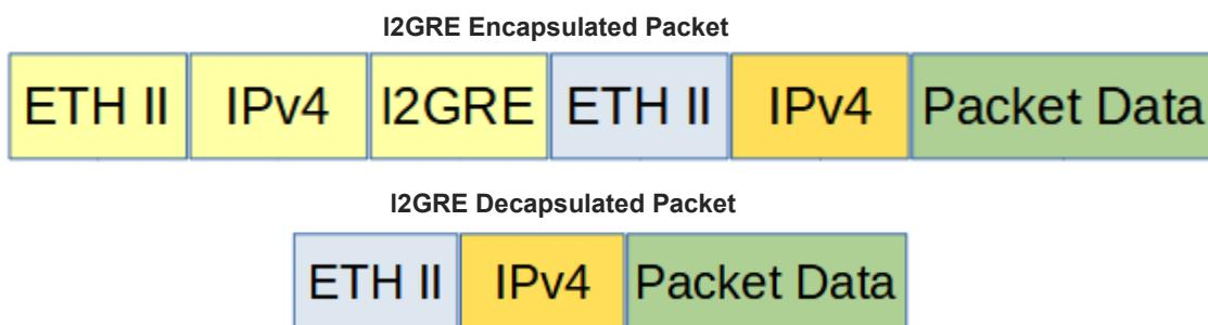
Decapsulating the I2GRE header from a packet(s) involves two configuration procedures.
