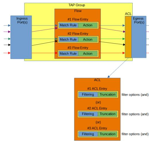
Also as shown in Figure 1, the entry filtering options are considered by the system as “and” options. Meaning for traffic to be permitted or denied, it must match all defined filtering options.
