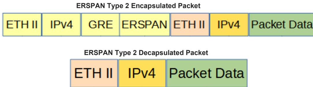
Decapsulating the ERSPAN Type 2 header from a packet(s) involves two configuration procedures.
