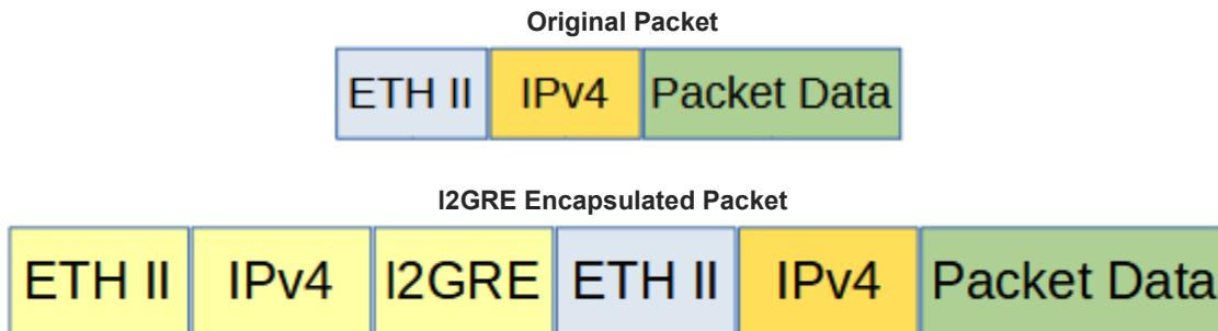
Encapsulating a packet with a I2GRE header involves two configuration procedures.
