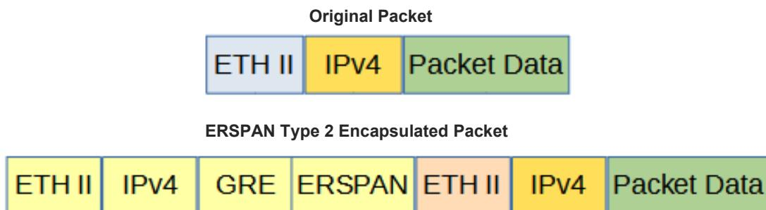
Encapsulating a packet with an ERSPAN Type 2 header involves two configuration procedures.
