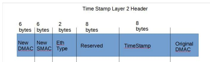
The time stamping is performed before the packet enters the switching chip. This function supports the standard Time of Day format and is accurate down to 8 nano-second resolutions. Software can distinguish
