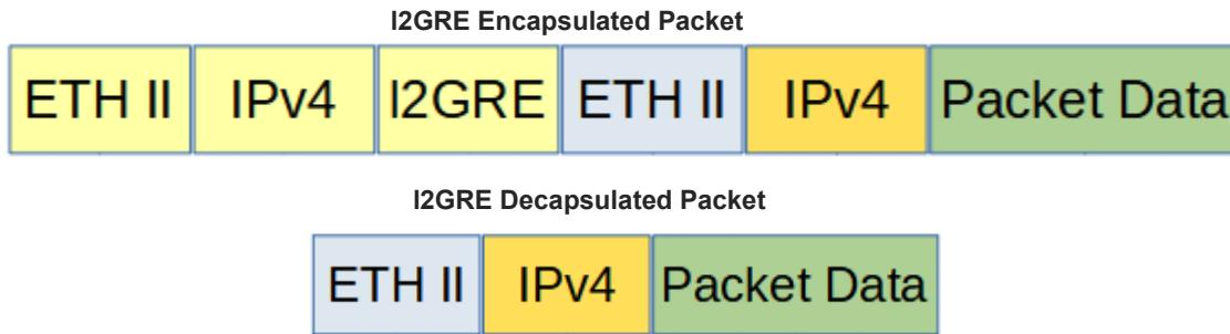
Decapsulating the I2GRE header from a packet(s) per VNI involves two configuration procedures.
