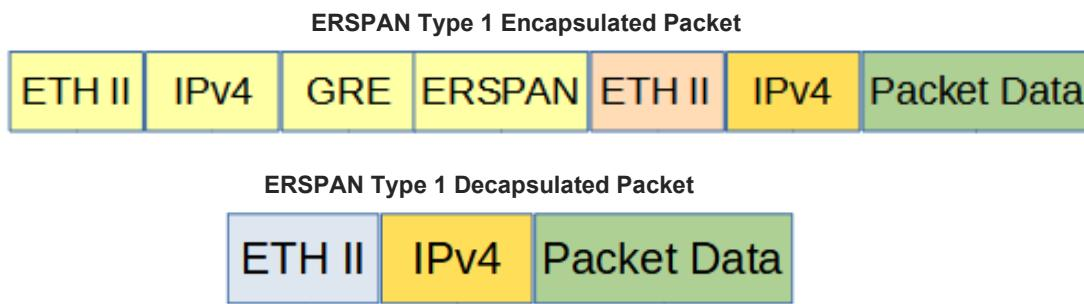
Decapsulating the ERSPAN Type 1 header from a packet(s) involves two configuration procedures.
