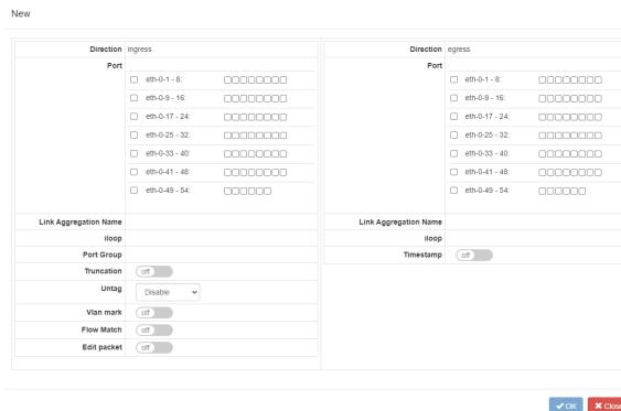
A screenshot of the 'TAP Group add detail' dialog box. It has two main sections: 'Direction: ingress' and 'Direction: egress'. Each section has a 'Port' list containing various network ports. Below each section are several configuration options: Link Aggregation Name, Untag (dropdown), Vlan mark (dropdown), Flow Match (dropdown), and Edit packet (dropdown). At the bottom are 'OK' and 'Close' buttons.
