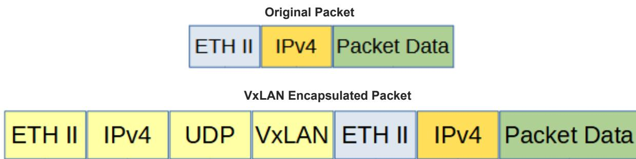
Encapsulating a packet with a VxLAN header involves two configuration procedures.
