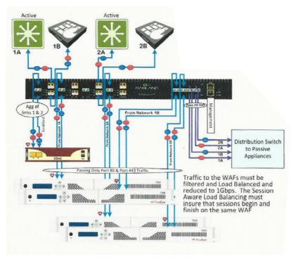
By combining the aggregation and load balancing with the tagging abilities of packet brokers all in one box, network architects can meet bandwidth demands without having to deploy extra equipment and making the network design more complex.
